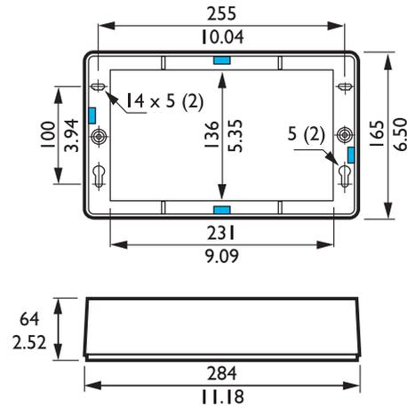
Dimensions in mm (in) with knockout boxes
